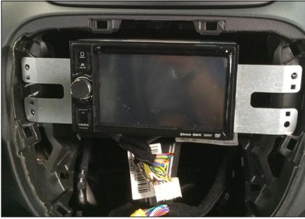
5. Connect all required circuit points and place double DIN head unit on dashboard. Fix head unit with original screws
