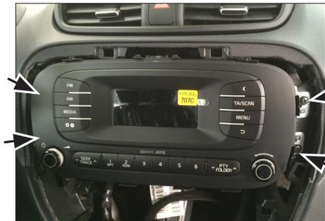
3. Remove all screws of OEM head unit
